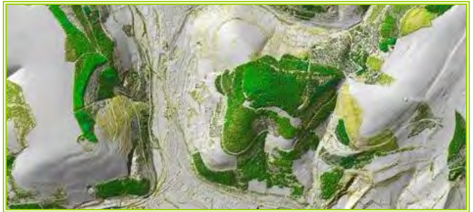
Part of the JPEG image of vegetation objects derived from LiDAR © Environment Agency
