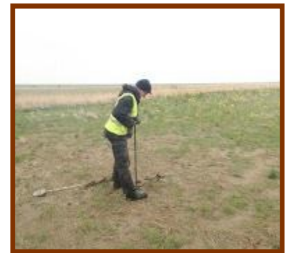
Figure 1 Hand augering during soil surveys
