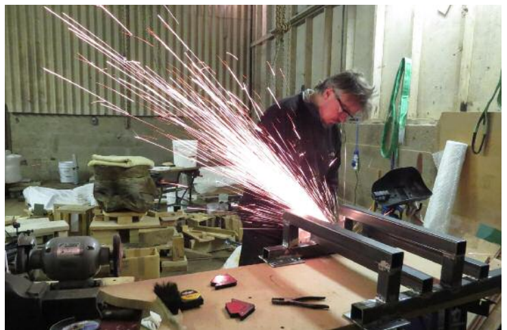
Making the welded steel mount on wheels to support the base of the trunk.
