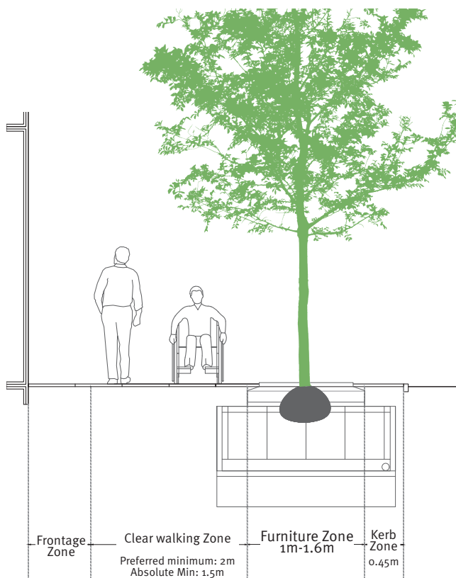
Figure 3. Fitting a SuDS Tree Pit into a street | Atkins
