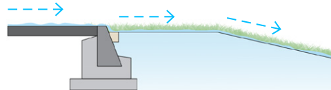
Using a filter strip to reduce pollutants
