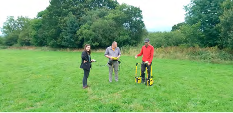
The use of ground penetrating radar and electrical resistivity tomography to study the subsurface structure of Ice Age ponds, has allowed reinterpretation of the mode of formation to include ground ice depressions linked to the interaction of permafrost and the retreating glacier, and potentially small pingos, as well as previously described kettle holes. Photo by Olivia Verplancke
