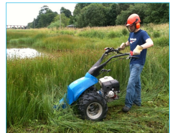
Photo to right: Volunteer using power scythe to cut rush around pool.
