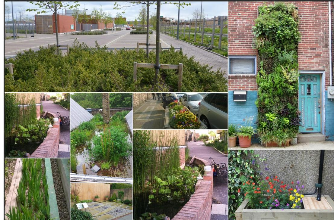
Raingardens are vegetated features which hold rain or surface water, slowly releasing it, helping to reduce the likelihood or severity of flooding.
